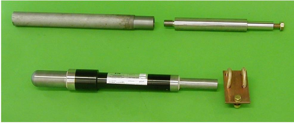
Dry molybdenum electrodes provide a cost-effective solution to applying direct electrical heating to glass. It is non-advancing and therefore should only be used in areas of low wear and modest temperatures, such as a forehearth. As the electrode is 'dry' there is no heat loss due to water-cooling.
