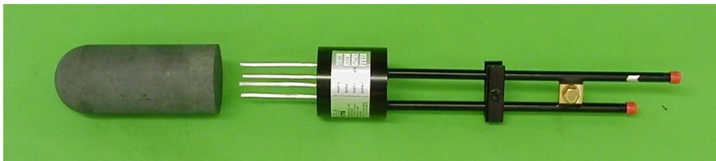
Tin oxide electrodes have been used for many years for the electric melting of glass. The main use is in heavily oxidised glasses, which would erode molybdenum electrodes, resulting in excessive molybdenum consumption and contamination of the product. On lead glasses tin oxide electrodes are usually used in the furnace, forehearth and gathering bay systems. For high quality soda lime glass tin oxide electrodes can be used in the forehearth and gathering bay systems.
