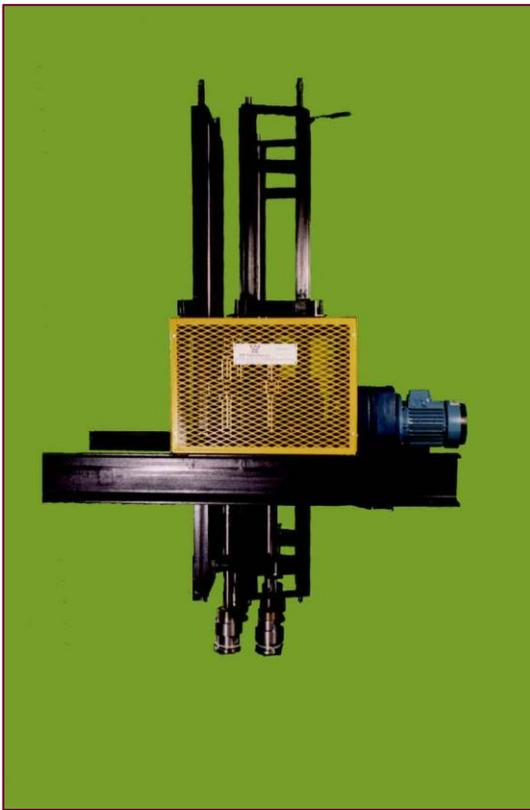
Forehearth stirrer assemblies are used to homogenise the glass in a forehearth or gathering bay by mechanically stirring the glass and breaking up any cord present in the system. They are used very effectively in lead crystal glass with up to 30% lead, particularly in reducing the effect of zirconia cord. Stirrers are essential in a colour forehearth to mix the frit with the base glass to ensure an even distribution of the colouring materials.
